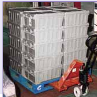
Products arrive at the distribution center in BinBoxes and go straight to the picking line — No Repacking; Pickers fill store orders from BinBoxes in flow racks. Empty BinBoxes are removed from the picking line for return to suppliers.
