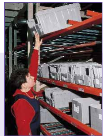
Products arrive at the distribution center in BinBoxes and go straight to the picking line — No Repacking; Pickers fill store orders from BinBoxes in flow racks. Empty BinBoxes are removed from the picking line for return to suppliers.
