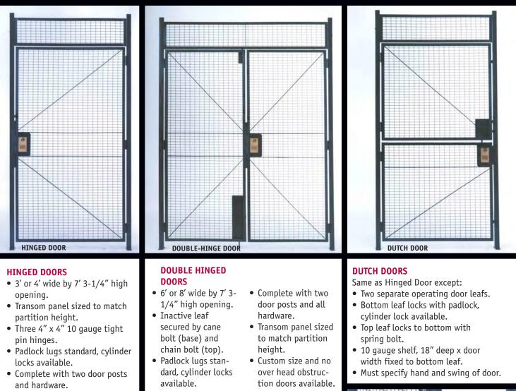
• Universal construction, works for left or right hand, inside or outside swing.
