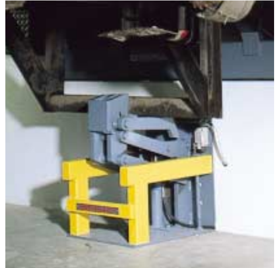
The restraining block of the Pentalock FM35 is shown in position on the truck’s ICC bumper.
