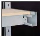
A heavy duty beam designed for greater capacity when used with deck material. Deck material sits on beam step and is supported by the appropriate number of Beam Brace/Heavy Duty Plywood Supports (order separately). Deck must be trimmed to 2" less depth than the depth of the upright frame.
