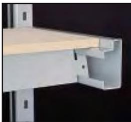
A heavy duty beam designed for greater capacity when used with deck material. Deck material sits on beam step and is supported by the appropriate number of Beam Brace/Heavy Duty Plywood Supports (order separately). Deck must be trimmed to 2" less depth than the depth of the upright frame.
