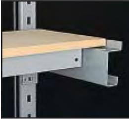
Designed to support 1/2" thick deck material flush with top of beam flange when used with the appropriate number of Plywood Support Angles which insert into slots in beam step. Overall height is 3-1/2". Beam step is 1-1/2" deep by 5/8" high. A 48" deep deck will fit between beams without trimming when a 48" deep upright frame is used.
