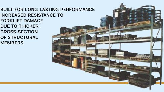
MECO OMAHA Structural Pallet Rack is designed in accordance with AISC and RMI Standards. Upright frames and load beams are fabricated from structural channel with a minimum yield of 36,000 PSI. Beams are secured to the upright frames with plated, heavy duty bolts and nuts - cannot be dislodged by forklift impact; installation is fast and easy with no special tools required.
