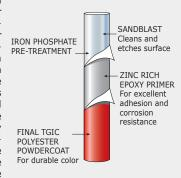
a hard shell that will protect the steel against corrosion and scratches. A final TGIC powdercoat is electro-statically applied and baked on to give the rack the final color and an additional layer of protection.
